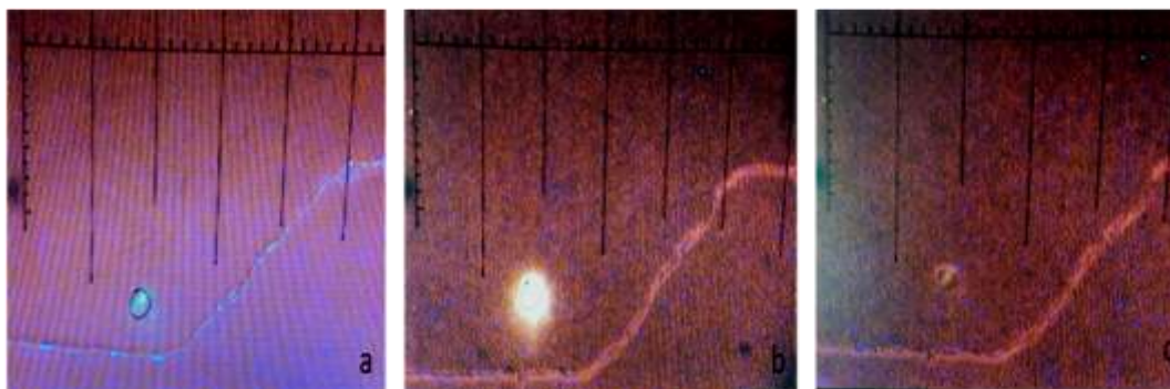
Fig. 6. Images of one P-gp expressing ovarian cancer cell (NCI/ADR-RES) retained in the cell retention structure of a microfluidic chip (a) after DNR (35 \mu\text{M} ) was added (at 200 s); (b) after CsA (5 \mu\text{M} ) together with DNR (35 \mu\text{M} ) were added (at 1400 s); (c) after trypan blue was introduced to treat the cell when the test ended (at 3400 s). After CsA was added together with DNR, the cell turns brightly fluorescent (b), and since the cell was not stained after the test (c), it was still viable after measurement. The times listed can be referred to in Figure 7 which depicts the measurement data. The scale was marked on the screen for cell size measurement, with the smallest graduation indicating 10 \mu\text{m} .
